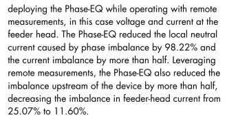
The third component of this project was to investigate diverse potential value streams from deploying the Phase-EQ for dynamic phase balancing. Relative to traditional utility solutions, device capabilities and benefits were considered in five technical areas: balancing phase voltage, balancing phase current, enabling higher DER penetration, reducing neutral current, and improving feeder efficiency. Additionally, approaches to monetize each value stream were proposed.
