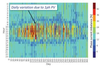
Plot illustrating time-varying phase imbalance exacerbated by single-phase solar systems
